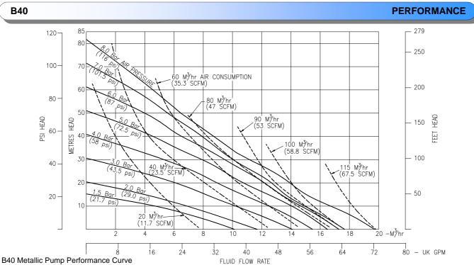
Performance based on water at ambient temperature
